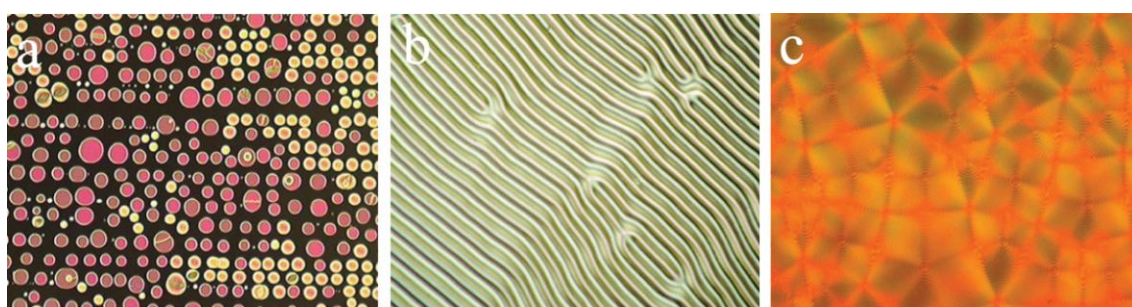
Figure 1.3 a) Texture of cholesteric phase b) Finger print texture of cholesteric liquid crystal c) Polygonal texture in cholesteric phase. (Adapted from source http://dept.kent.edu/spie/liquidcrystals/textures2.html ).
