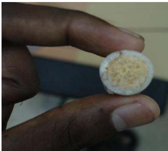
Figure 4.8. Snapshot of polyacrylamide sample showing the formation of yellowed core (due to imidization) and outer polymer skin formed due to polymerization of evaporating monomer vapors
