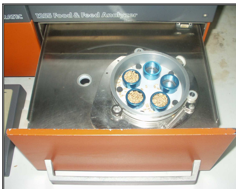
Fig. 2.4: The samples filled in the sample cups of Infrared analyzer 300 (Technicon, NY, USA)
