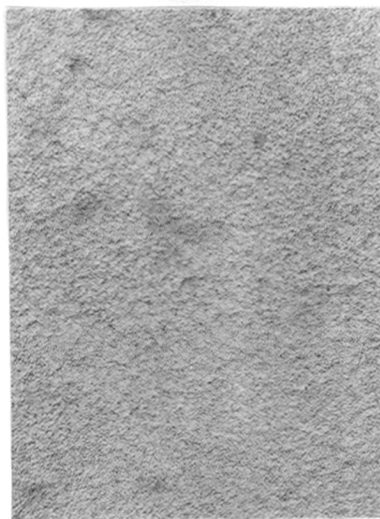
Fig.30. Silver deposited from thiosulphate bath at 5 mA/cm 2 and 20°C. x 600.
