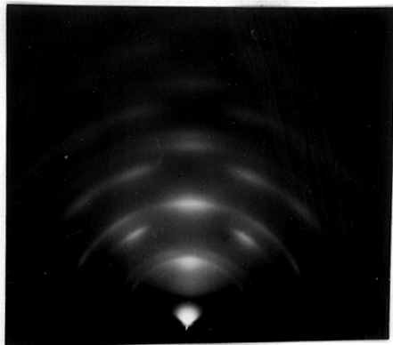
Fig.21. Silver deposited from cyanide bath with carbonate addition at 10 \text{ mA/cm}^2 and 20^\circ\text{C} . (10\bar{1}0) orientation.
