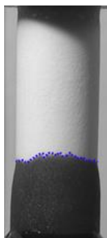
Figure 5.7: The jagged growth front of the colored water front, as it propagates, is averaged and the height of this growth front from the water surface is determined. Here, the front is shown as a blue dotted line.
