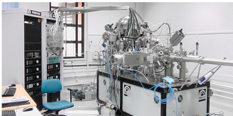
Figure 2.6: A photograph of NAPPES unit at CSIR-NCL.
