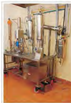
Schematic experimental setup for continuous synthesis of pure lactic esters using high pressure reactor (10 L capacity)
