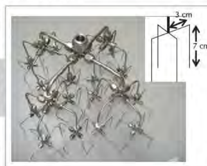
Fig. 1: The 64 channel network in vertically downward orientation. Inset: schematic of a single split
