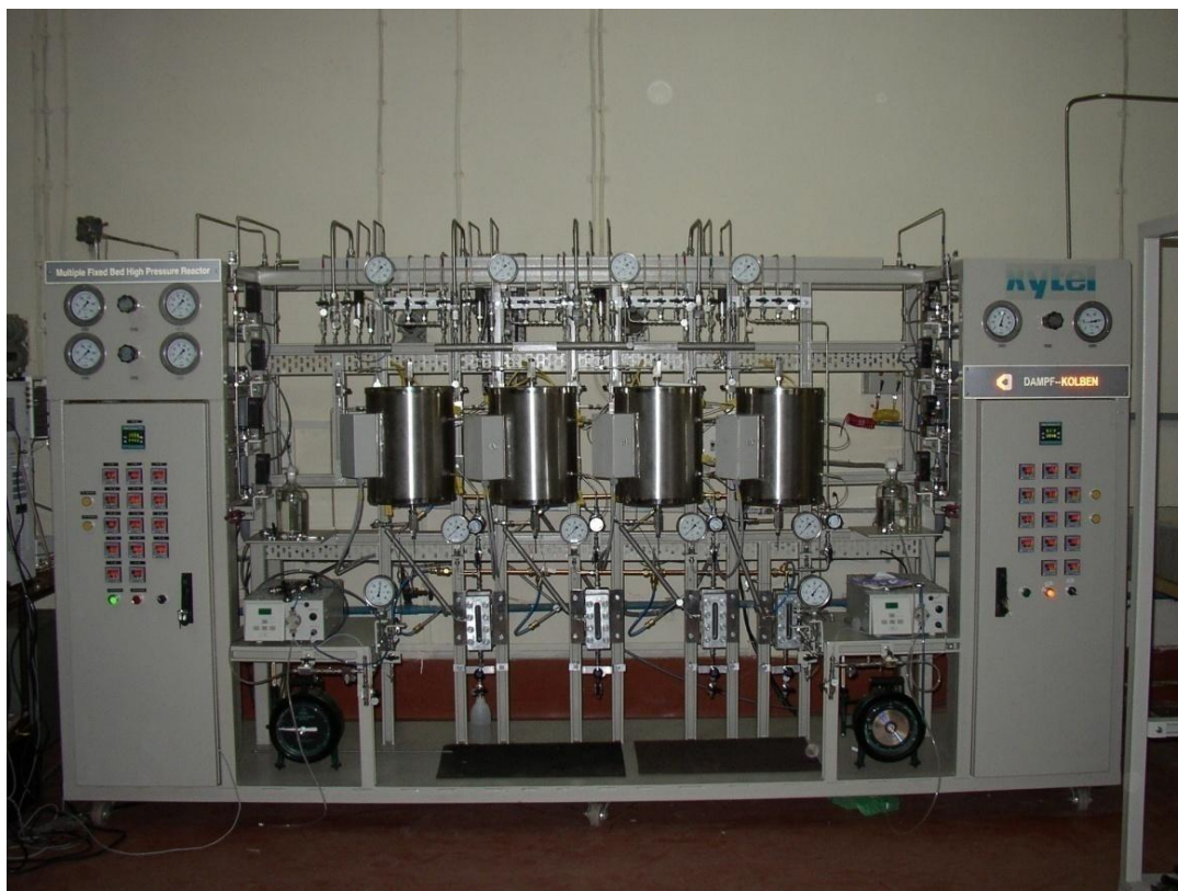
Fig. 2.9. Multiple fixed bed reactor used for testing the catalysts
