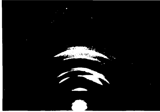
Fig. 46. HgTe on (110) NaCl deposited at \sim 100^\circ\text{C}
