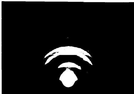
Fig. 57. \text{In}_2\text{Te}_3 on glass support deposited at \sim 300^\circ\text{C}
