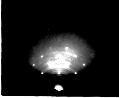
Fig. 42. HgTe on (110) NaCl deposited at \sim 80^\circ\text{C} Beam along \langle 001 \rangle
