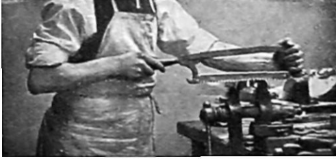
FIG. 17.—Method of holding a hack saw.
