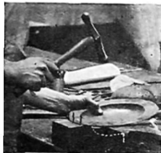
FIG. 2.—Raising a dish on a wood mould.
