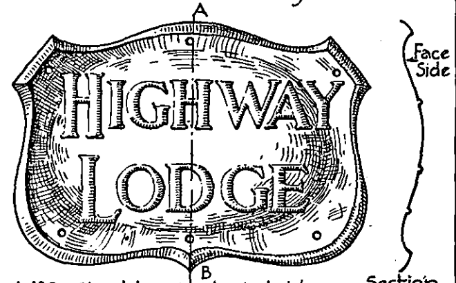
N°2. Shield raised first then the letters raised on shield
