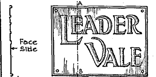
N°3 letters raised from flat ground & border raised
