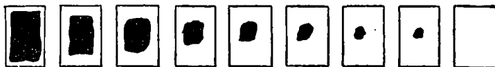
FIG. 77.—Showing progressive diminution of a dark core on prolonged heating in air.
