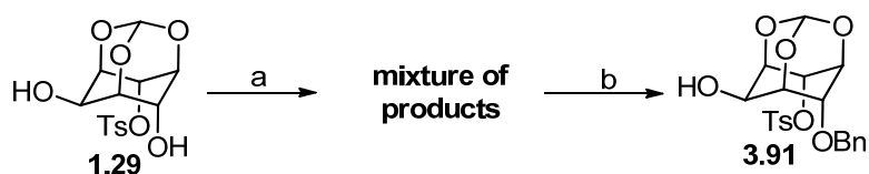
Scheme 3.4: (a) DMF, 3.0 equivalent NaH, 3.5 equivalent BnBr; (b) column chromatography.
