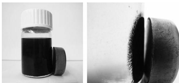
Fig. 3.23. Magnetic separation of finely dispersed \text{SO}_3\text{H-MS} catalyst
