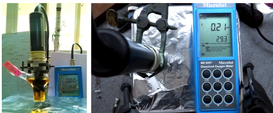
Figure 3.5: Experimental set-up (left) for the determination of dissolved oxygen produced as a result of reaction of [Ru(bipy) 3 ] 3+ (4 eq; 0.84 mM) with a well-defined Fe V (O) (right).
