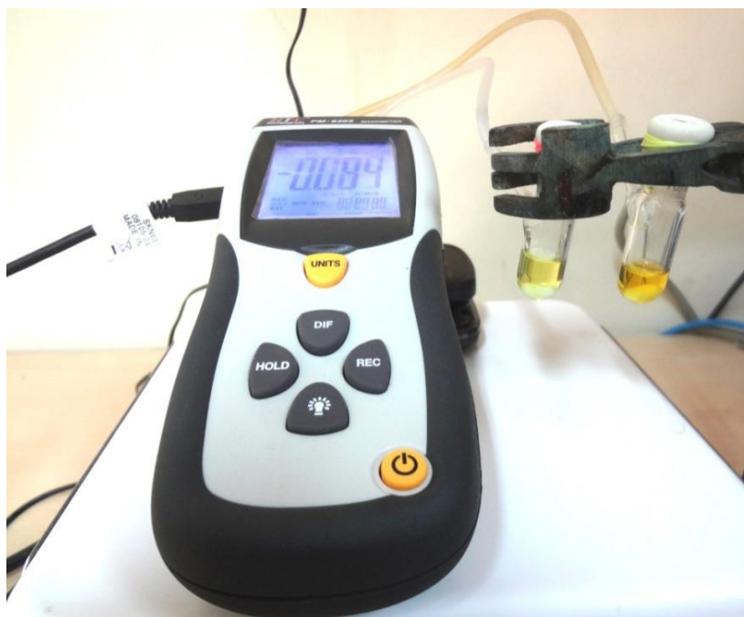
Figure 3.2: Two port sensing approach for monitoring differential pressure increase in the reaction vial (left) with respect to the reference vial (right) by a manometer at 25 °C.
