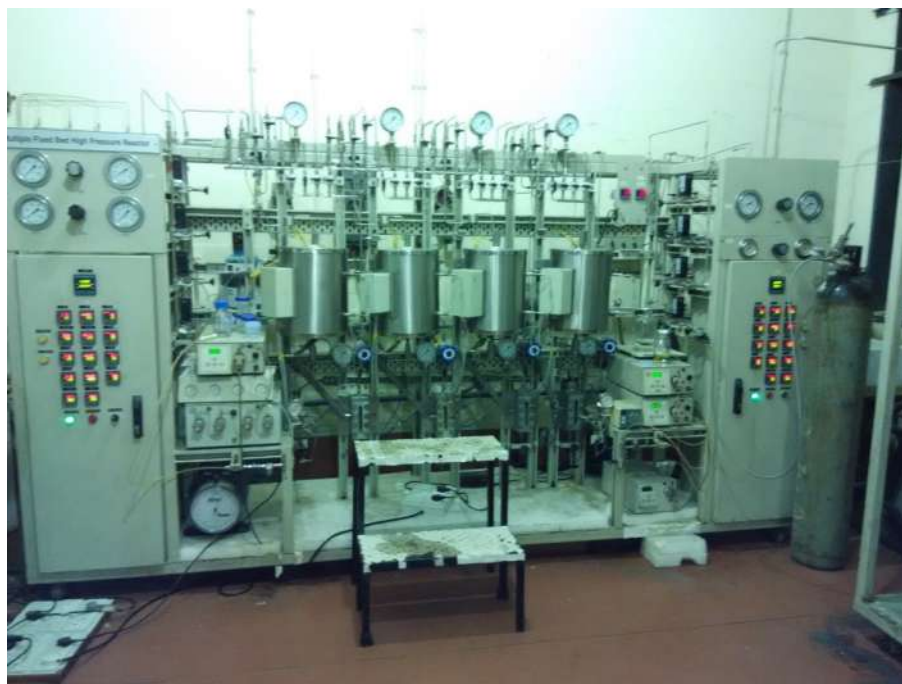
Figure 1. Multi fixed bed flow reactor on which ethylbenzene to styrene with Mn_xTi_{1-x}O_2 catalysts were studied.
