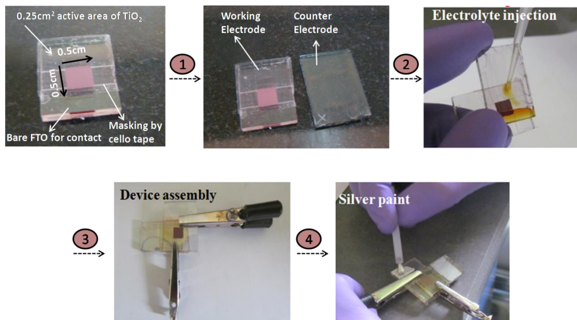
Figure 2.5. Visual photographs of steps involved in assembling DSSC device for testing its photovoltaic performance.
