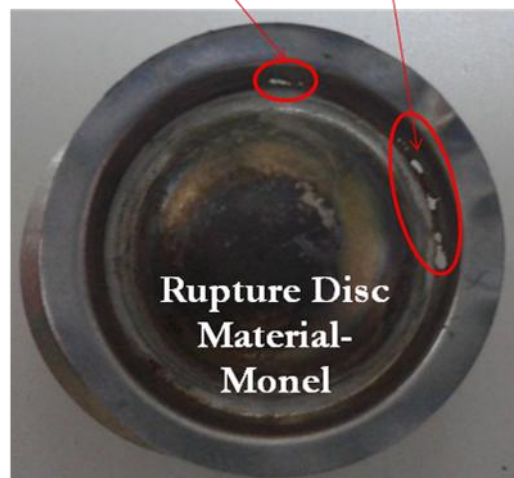
Figure 3.11. Image of rupture disc, damaged by the action of SO 2
