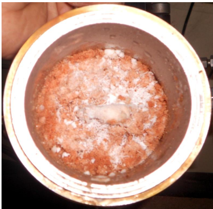
Figure 5.2. Methane hydrates in silica sand (Brown=silica sand, white=hydrates)
