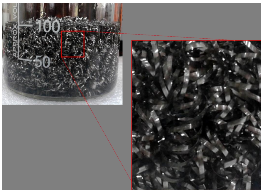
Figure C1: A representative photograph of the SSP-1 (SS-316) random packing
