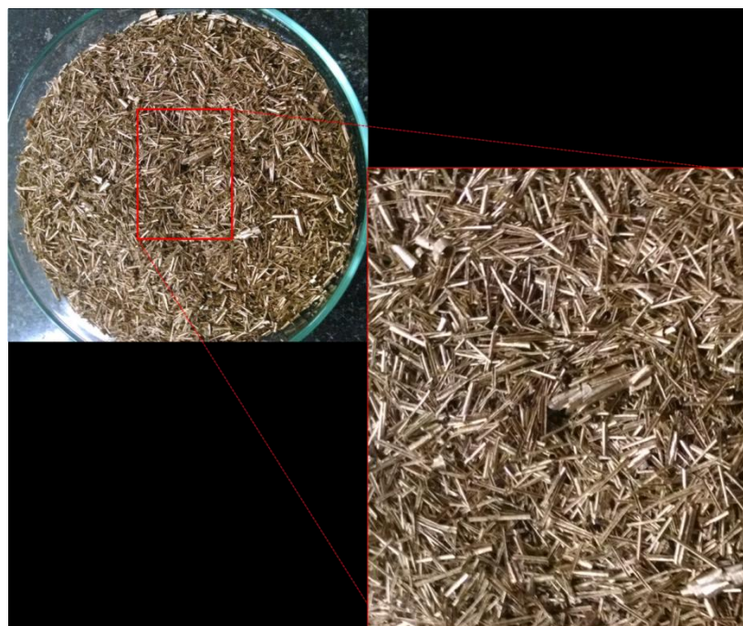
Figure C4: A representative photograph of the brass packing used in this study
