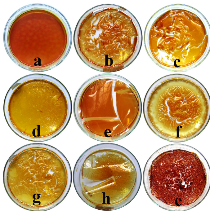
Figure 5.6 Photographs of PILs (a) [DBzDMPBI-BuI][I], (b) [DBzDMPBI-BuI][Gly], (c) [DBzDMPBI-BuI][L-Ala], (d) [DBzDMPBI-BuI][L-Arg], (e) [DBzDMPBI-BuI][L-Asp], (f) [DBzDMPBI-BuI][L-His], (g) [DBzDMPBI-BuI][L-Lys], (h) [DBzDMPBI-BuI][L-Phe] and (i) [DBzDMPBI-BuI][L-Try].
