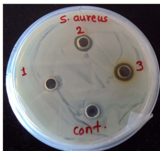
Figure 3.14: Antibacterial activity of Ag-NPs embedded 1-PAm, 2- PAm:PAS (80:20), 3- PAm:PAS (50:50) compared with Control- Pure hydrogel
