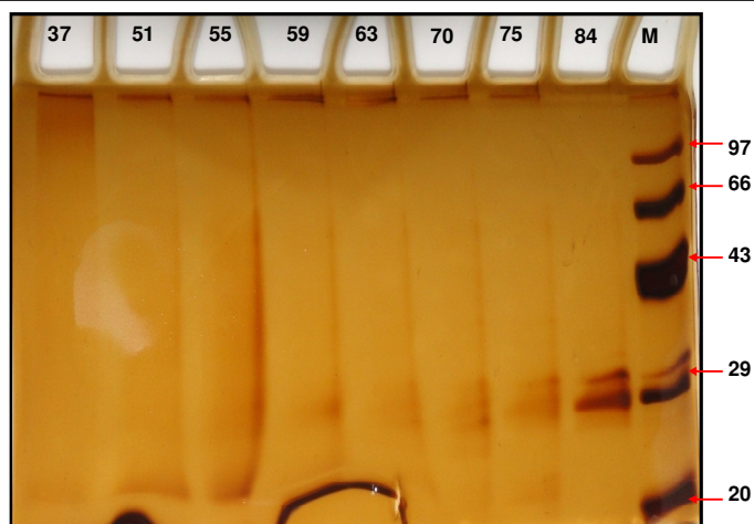
Figure 4.9: SDS PAGE gel electrophoresis of fractions collected from FPLC which were showing high activity in formation of nanoparticles. Fraction 37 showing no protein band, where the activity was absent, 51 and 55 fractions showing 21kDa proteins. Fractions 59 to 84 showed 29 and 30kDa protein.
