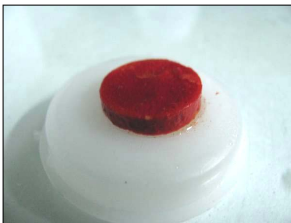
Figure 4.33 : Pictorial representation of St-DVB polyHIPE containing cadmium sulphide (CdS) particles
