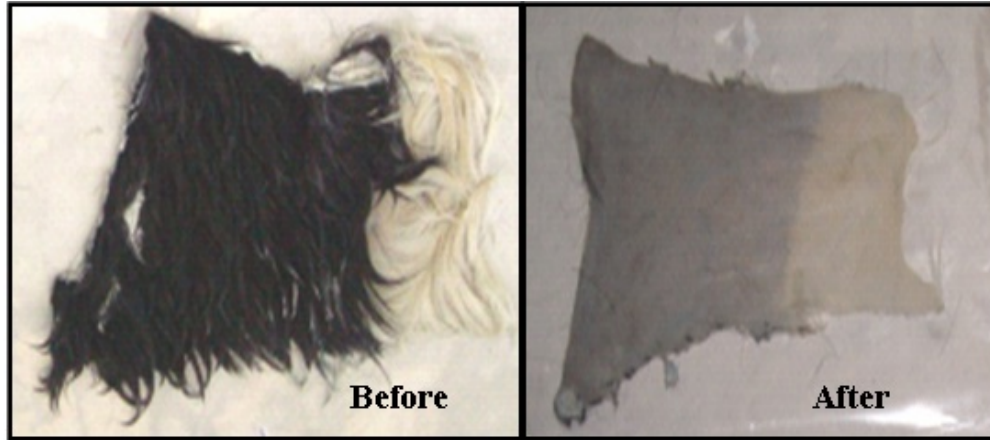
Figure 4.1.6: Dehairing of goat skin with lime and sulfide
