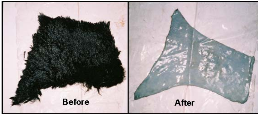
Figure 4.1.9: Dehairing of sheep skin with lime and sulfide
