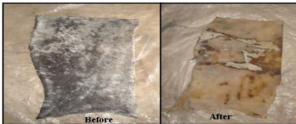
Figure 4.1.11: Dehairing of cow hide with lime and sulfide
