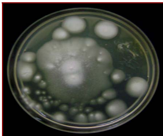
Figure 2.4.11: Plate assay for lipase activity
