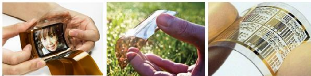
Figure-1.1. Flexible OLED display technology driven by organic transistors (left) [adapted from http://www.sony.net/SonyInfo/technology/technology/theme/8ido18000001prgv-img/8ido18000001prpz.jpg ], plastic solar cells (middle) [adapted from http://www.aps.org/publications/capitolhillquarterly/201302/whatsnewininnov.cfm ] and organic integrated circuits (right). [adapted from NPG Asia Materials research highlight ; doi:10.1038/asiamat.2011.48]
