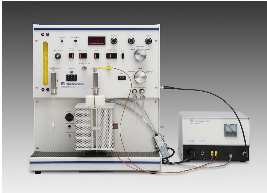
Figure 2.7. Chemisoft TPx (Micromeritics-2720) instrument
