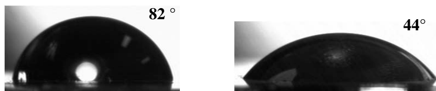
Figure 6b.3 Water droplet on polyamide PPA-2 (a) before and (b) after PEG 550 grafting
