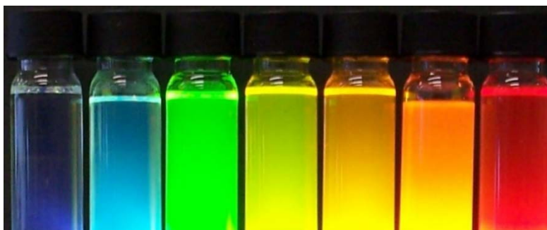
Figure 1.3. Emission from CdSe QDs of varying size (size increases from left to right). [19]
