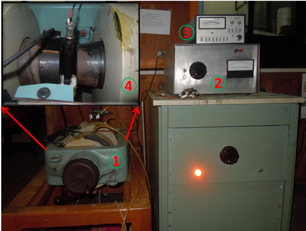
Figure 2.8. The experimental setup used for thermal conductivity measurements in the presence of a DC magnetic field, (1) Electromagnet, (2) DC power source, (3) gauss meter, (4) the fluid sample in a test tube located between the pole pieces of the electromagnet.
