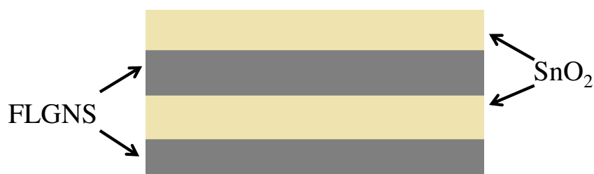
Scheme 2.2 Schematic representation of SnO 2 /GNS composite.
