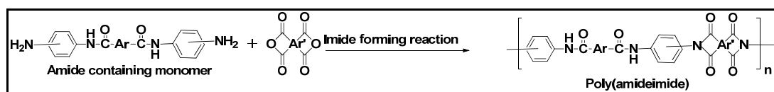
Scheme 1.13 Imide forming reaction using amide containing monomer
