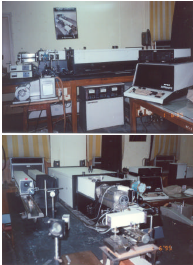
Fig. 2.8 The Schematic Diagram and Photograph of the Laser Raman Setup
