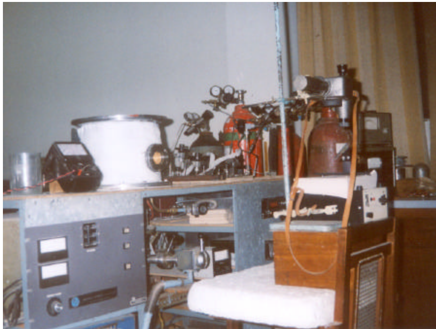
Fig. 2.1 The Schematic Diagram and Photograph of the HF-CVD System used for the deposition of the diamond films
