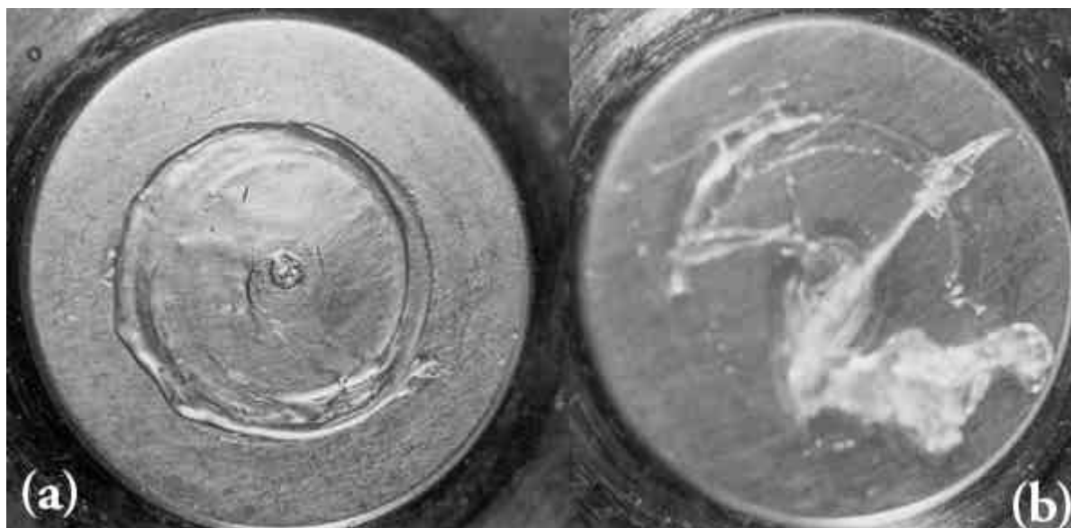
Figure 5.3 The photograph of the plate immediately after the instability has occurred in the cone and plate rheometer. The left picture (a) is from the plate where the coated cone was used, while the right picture (b) corresponds to a bare cone. The sample with the coated cone is almost free from distortions relative to the bare cone case.
