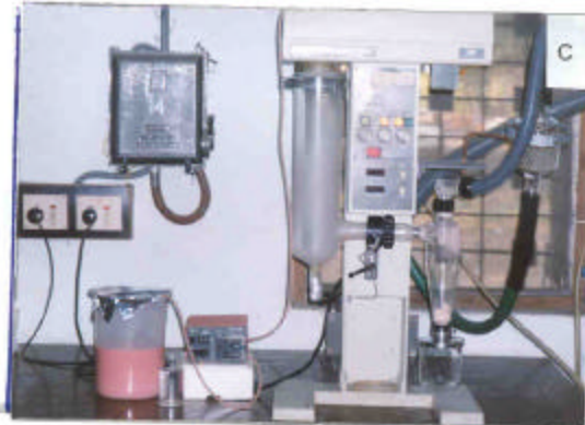
Figure 8.2 Step wise feed preparation from Rhodotorula glutinis NCIM 3353 [A. Fermentation, B. Microfiltration and C. Spray drying].
