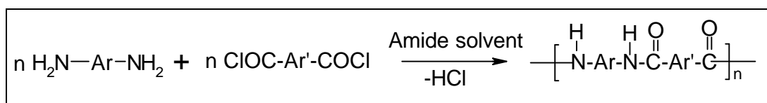
Scheme 1.1. Solution polycondensation of diamine and diacid chloride
