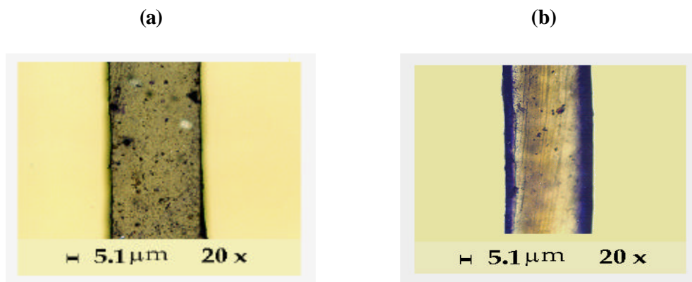
Figure 3.12 Effect of solvent (acetone + toluene) on thickness of grafted layers of HEMA onto EPDM film surface for photo-grafting carried out at R.T (a) 1.0 M and (b) 2.0 M.
