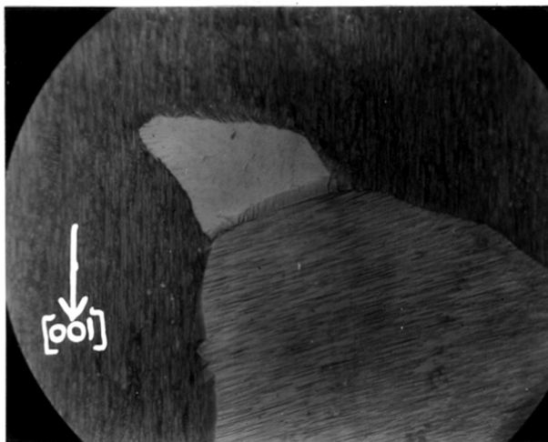
Figure 57. Micrograph of 22,000 Å. deposit on Fe (110) face from chloride bath at 70°C. and 11 mA./sq.cm.
