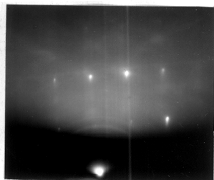
Figure 3. Ag deposited on Fe approx. (001) face from N/2 AgNO_3 at 1 \text{ mA/cm}^2
