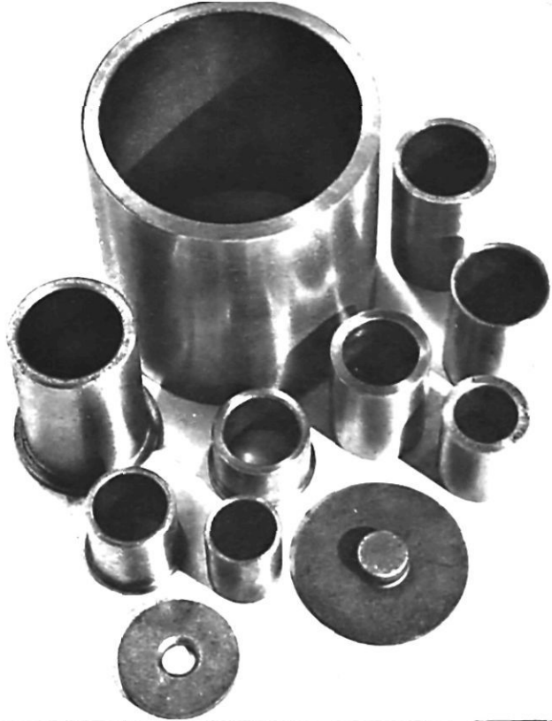
Above. Moulded bearings produced from copper powder mixtures. Below. Left: Steel component with bush formed from bronze strip. Right: Hot brass stampings for carburettor levers.
