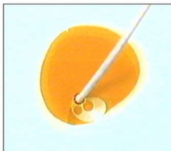
Fig.4.10: Image of the viscous fingering pattern formed at a particular instant during injection of chloroform containing AOT (colored phase) into an aqueous solution of SrCl 2 and Na 2 CO 3 .
