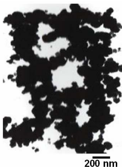
Figure 5.7: TEM picture of the UV-irradiated PTA–Ag nanoparticle solution after alkali treatment.
