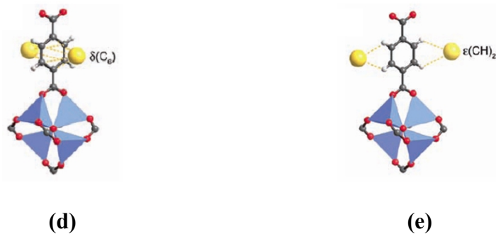
Figure 5: Schematic representation of the symmetry-independent sites, partially occupied by Ar atoms, at 30 K (shown as yellow spheres) in the pores of MOF-5.
