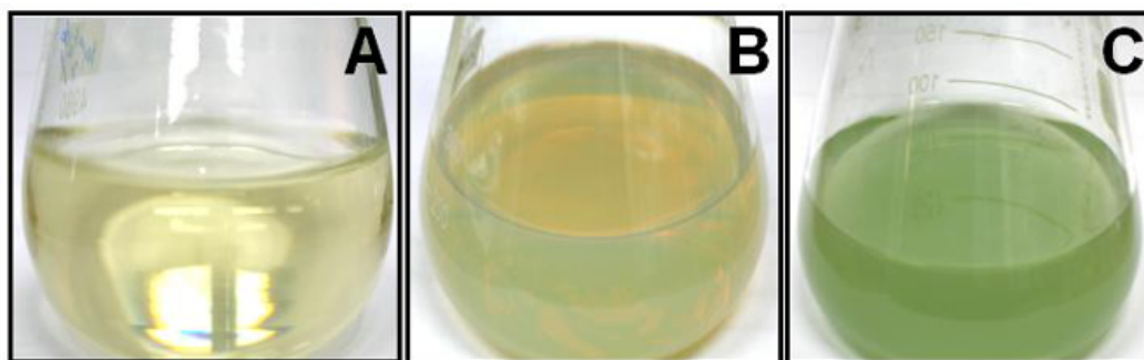
Figure 4.19 Changing colour of the silver nanoparticles synthesized by modified seedless surfactant less protocol of Murphy [50] as a function of time (12 h, A; 48 h, B; 5 days, C) indicating the evolution of the triangular morphology.
