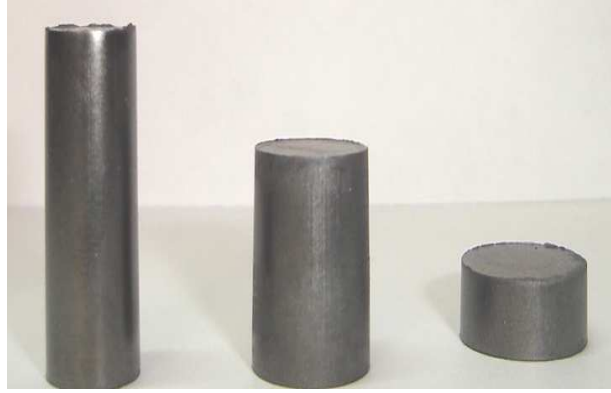
Figure 2.4: Different shapes of cobalt ferrite samples used for magnetostriction measurements.
