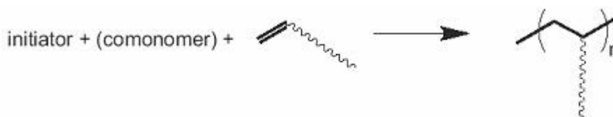
Figure 6.2: Synthetic approaches for graft copolymers
