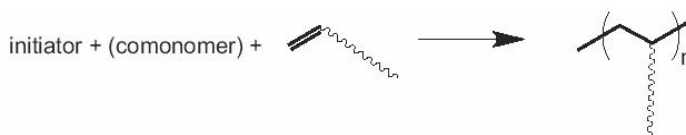
Figure 1.12: Graft copolymer by grafting through approach
