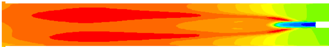
Figure 6.7b: Temperature contours in central vertical plane of freeboard region, K
