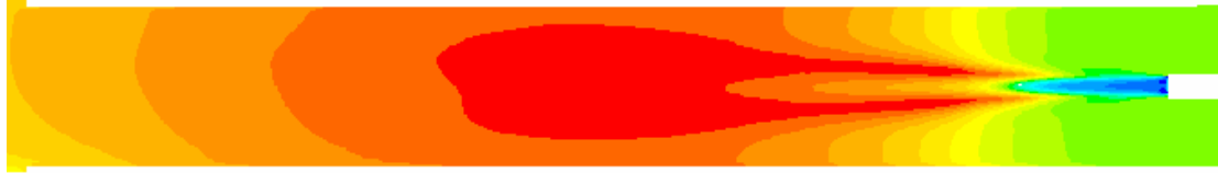
Figure 6.7a: Temperature contours in central vertical plane of freeboard region, K
