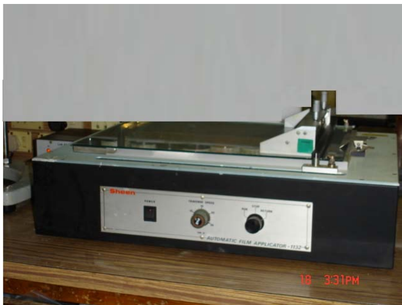
Figure 5.1 Sheen automatic film applicator.
