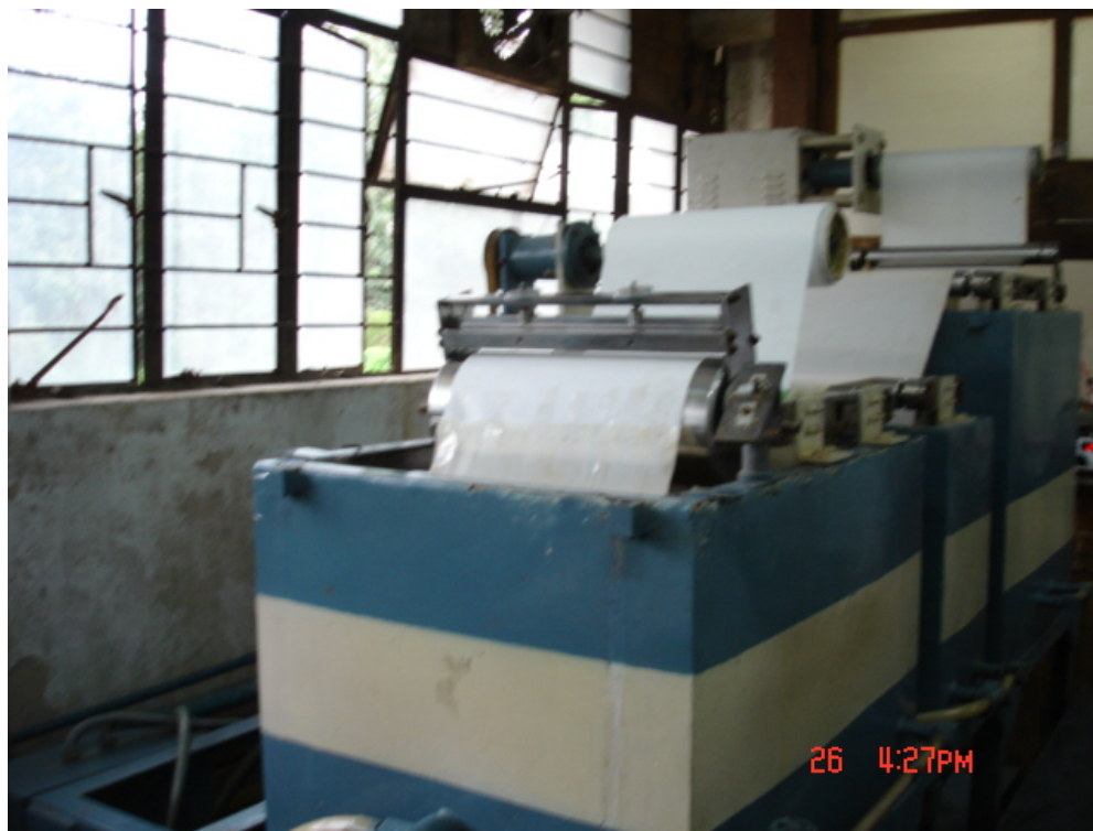
Figure 3.1 Continuous membrane casting machine.
