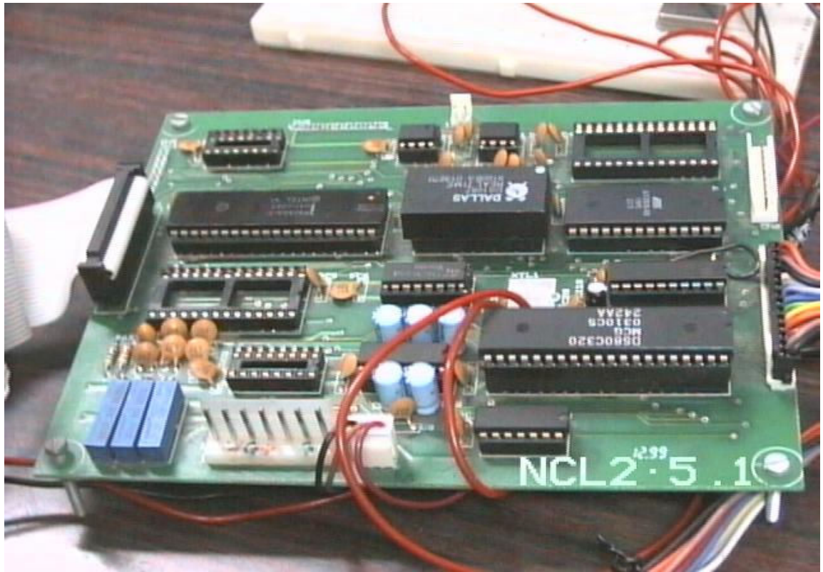
Figure 3.4-II -Developed board for 80C320 microcontroller hardware
