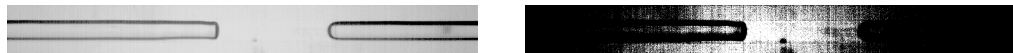
Figure 2.5 (a) Channel (inner) diameter not visible in water-glycerol/nitrogen system (b) channel (inner) diameter made visible on contrast adjustment
