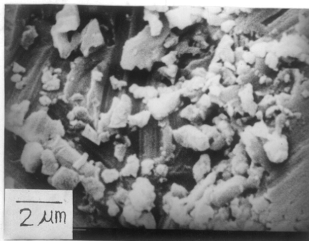
FIG. 5 : Scanning electron micrograph of Sample C-1 (heated at 950°C)
