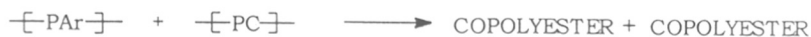
Scheme 1.23 : Possible interchange reactions between poly(aryl carbonate)s and poly(aryl ester)s during melt blending process.
