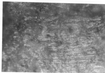
Figure 3.15 Optical micrograph of the melt extruded PP-CaSO 4 samples sectioned parallel to the extrusion direction taken in reflection mode from top surface. (net magn. = 450x)
