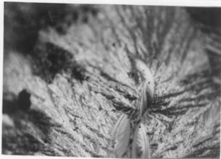
Figure 6.22 Optical micrographs for PMMA-PNA (SC) films containing (a) 30% (b) 40% and (c) 45wt.% PNA respectively . (net magn.= 450x)
