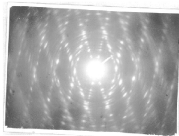
Fig. 113 Sb_2S_3 on NaCl (100) at 350°C
