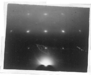
Fig. 72 CuCl on NaCl (110) at 200°C beam along \langle 001 \rangle
