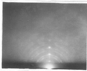
Fig. 52 CuBr on NaCl (100) at 150°C.
