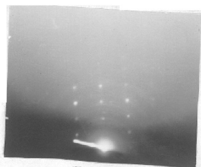
Fig 59 CuBr on NaCl (111) at 200°C.
